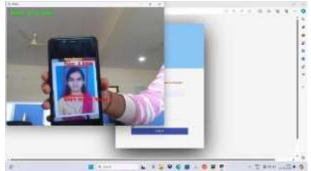
Fig. 5.4. The system successfully detecting and rejecting a spoofing attack.
