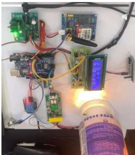
Fig. 1. Assembled hardware prototype: Arduino UNO (center), PZEM-004T (left, green board), SIM800L GSM (right, blue board), NodeMCU, relay module, I2C LCD displaying V:236 Cr:0.42 Tf:27 Gr:1, and Philips bulb as test load.
