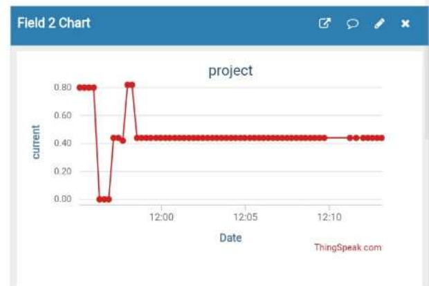
Fig. 3. ThingSpeak Field 2 (Current) chart: 0.42 A steady-state following initial transient settling.
