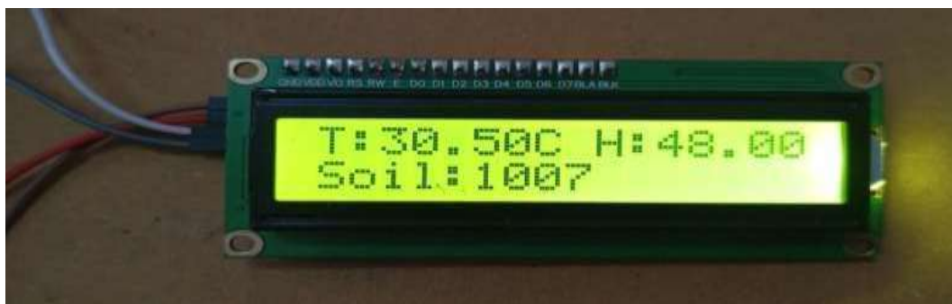
Fig.2: Output of Arduino based automation system
