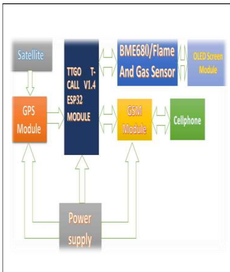
Fig.1 Block diagram of ESP32 based vehicle tracking system.
