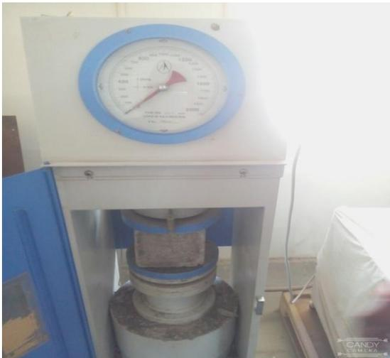
**Fig-5: Compression testing machine**
