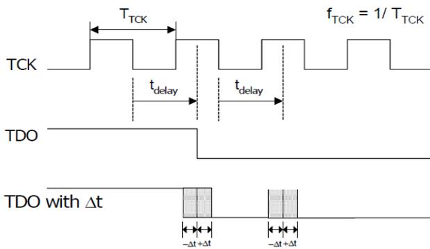
Fig -5: Timing Diagram for TAP Signals
