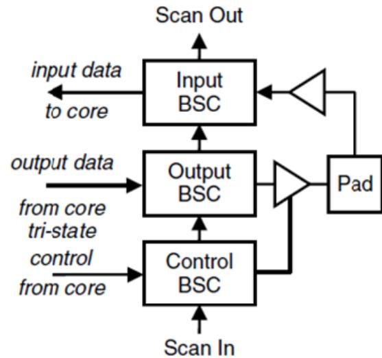
Fig -4: Bidirectional Buffer with multiple Boundary Scan cell
