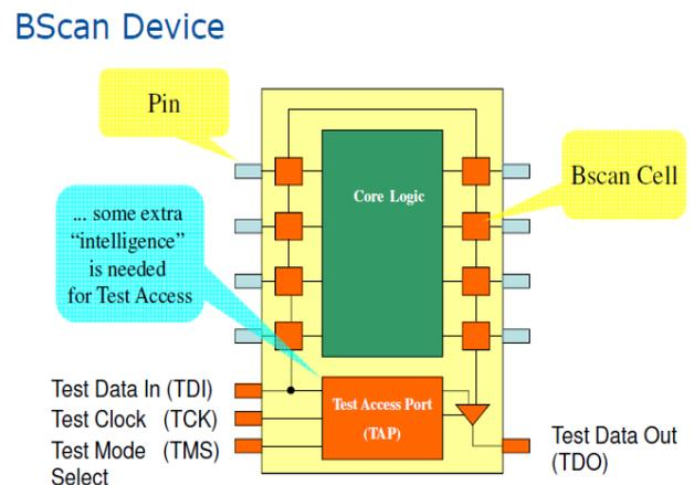
Fig -2: Boundary Scan Device
