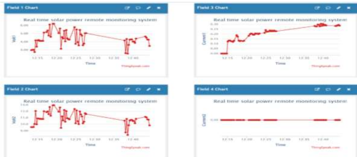
Fig.5(b) Recorded data in the morning (Field1)Voltage1 Vs Date/Time graph,(Field2) Voltage2 Vs Date/Time graph,(Field3) Current1 Vs Date/Time,(Field4) Current2 Vs Date/Time.
