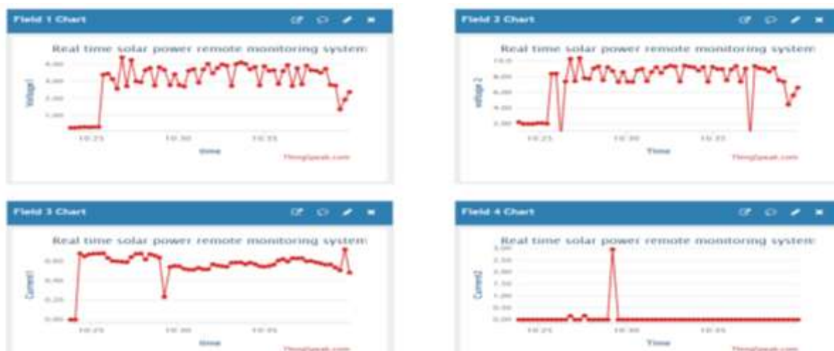
Fig.5(a) Recorded data in the morning (Field1) Voltage1 Vs Date/Time graph, (Field2) Voltage2 Vs Date/Time graph, (Field3) Current1 Vs Date/Time, (Field4) Current2 Vs Date/Time.
