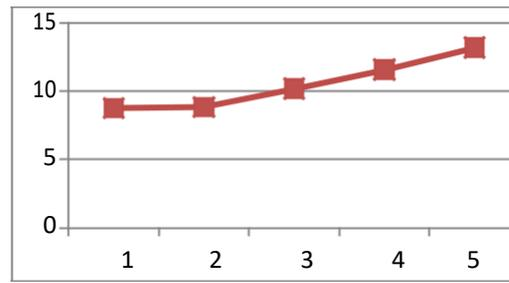
Fig. 6. Impact of biscuit loading on water sorption of LAC with fifty wt.% CW. . X axis levels of biscuit% Y axis absorption %
