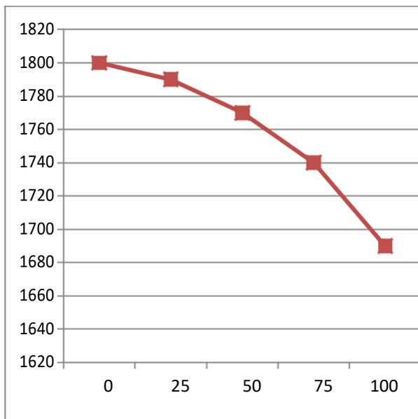
Fig. 5. Impact of levels of biscuit on bulk density of LAC containing fifty wt.% of CW with distinction levels of biscuit replaced FAM. X axis levels of biscuit% y axis Bulk density kg/m<sup>3</sup>
