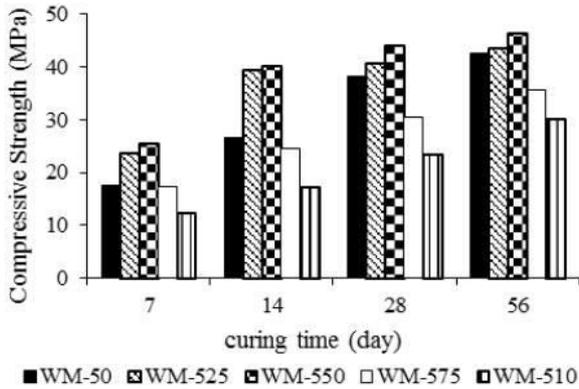
Fig. 4. Compressive strength of LAC containing fifty wt.% of CW with distinction levels of biscuit replaced FAM.
