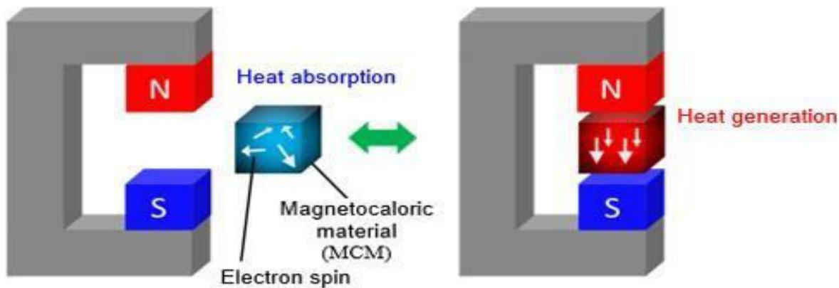
Fig.2: Magneto-caloric effect
