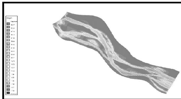
Below shows the bathymetry developed for Sarada river using delft3D.
