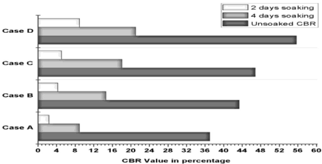
This study demonstrates that the application of Medium Setting (MS) bitumen emulsion can significantly enhance the California Bearing Ratio (CBR) of subgrade soil when proper mixing and curing are implemented. Optimal results are achieved when the soil-emulsion mixture is allowed to cure for approximately five and a half hours post-mixing.
