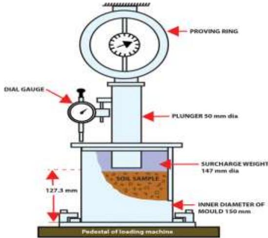
Fig. 3.2:- California Bearing Ratio Testing Machine
