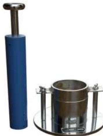
*Figure 3.1:- Modified Proctor Test Apparatus*
