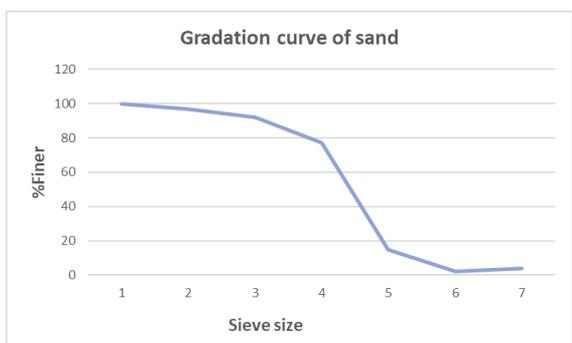
**Fig 4: Particle size distribution curve of Sand**
