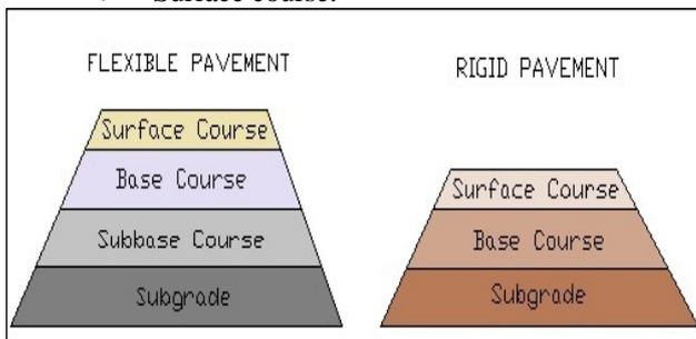
**Fig1: Components of Pavements**
