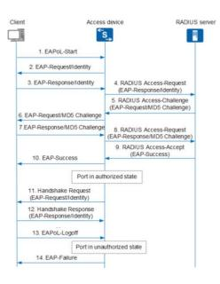
Figure 2.1: Sequence Diagram showing Dot1x authentication
