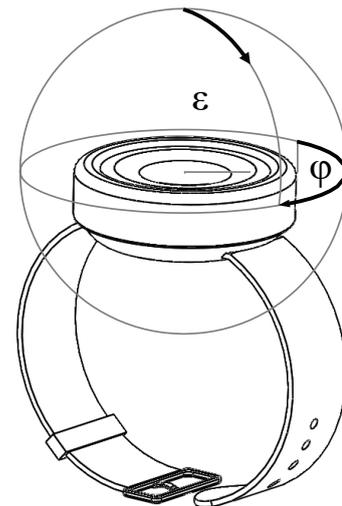
Fig..Schematic representation of the co-ordinate system.
