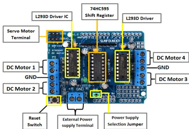
**FIG 5.1 L293D Motor Driver**
