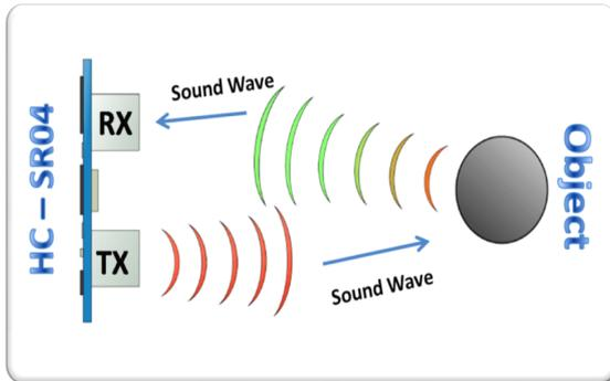
**FIG:5.2 Ultrasonic Sensor**
