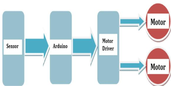
FIG 3.1 Block Diagram of Line Following Robot
