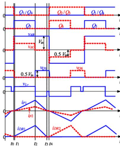
FIGURE 2. Key waveforms of the proposed converter.
