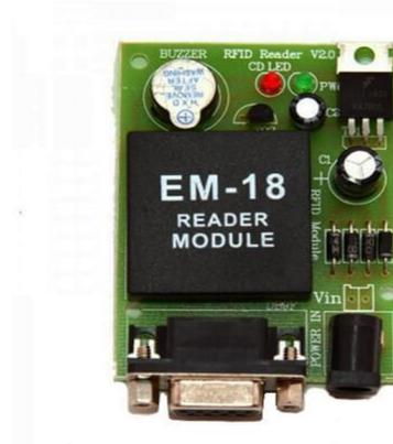
Fig -3: RFID Tag reader
