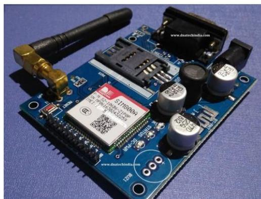
Fig -5: GSM Module
