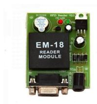
Fig -3: RFID Tag reader
