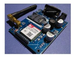
Fig -5: GSM Module
