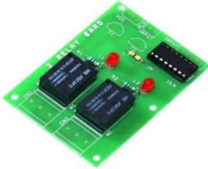
Fig 5: Two Relay board
