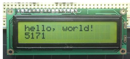
**Fig -6: Liquid Crystal Display**
