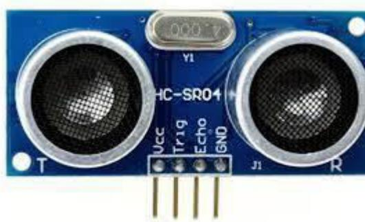
**Fig -2:** Ultrasonic Sensor
