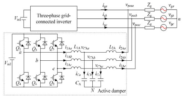
Fig. 2 Circuit Diagram of Three phase grid connected inverter with adaptive active damper
