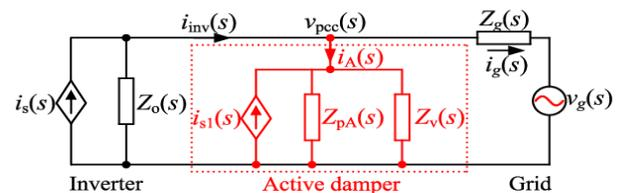
Fig.1 Active Damper System Connection
