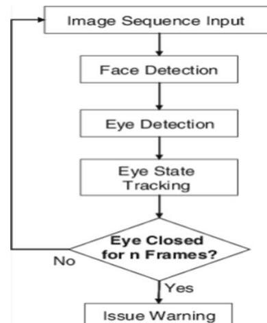
Fig. 1 Flow chart drowsiness detection and alerting
