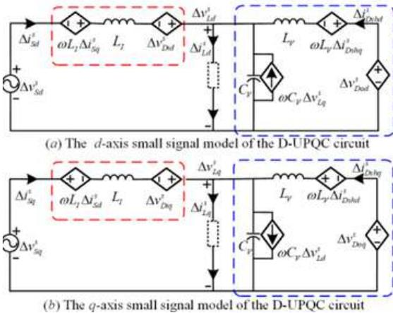
FIGURE5. The dq-axis small signal model of the D-UPQC circuit.
