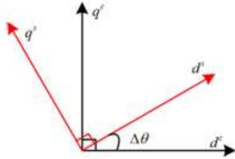
FIGURE2. The system and control frames.
