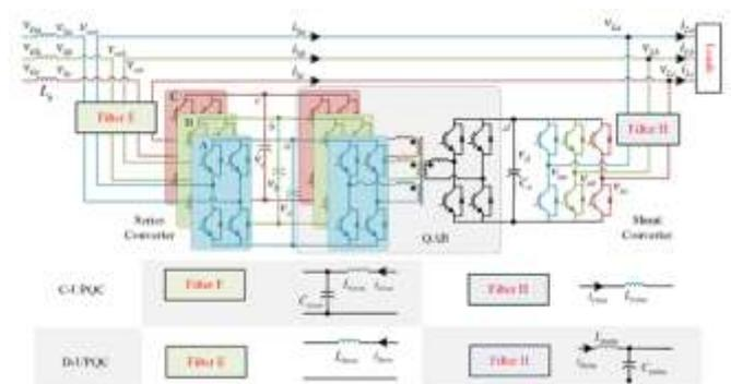
FIGURE 1. Configuration of three-phase UPQC-QAB.
