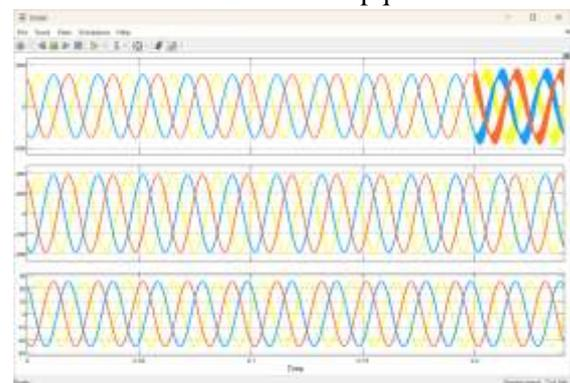
Figure 23. The simulation waveforms under high-frequency grid voltage harmonics distortion: Multi upqc
