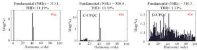
FIGURE 16. The spectrum analysis of vSa and vLa under high-frequency grid voltage harmonics distortion. The load voltage in the C-UPQC is mostly distorted by harmonics; in two schemes, the load voltages are distorted by the load current harmonics.
