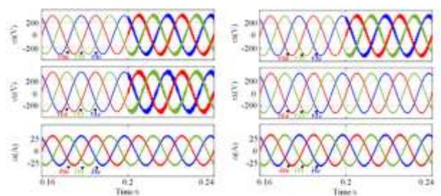
FIGURE 15. The simulation waveforms under high-frequency grid voltage harmonics distortion: (a) C-UPQC, (b) D-UPQC.
