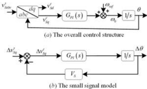
FIGURE3. The control block diagram of the SRF-PLL
