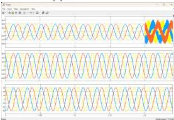
Figure 25. The simulation waveform under different grid impedance: Multi UPQC.
