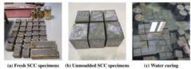
Fig. 2. Representative specimen preparation and water-curing stages.
