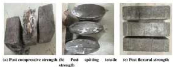
Fig. 6. Representative post-test failure patterns: compression, split tension and flexure.
