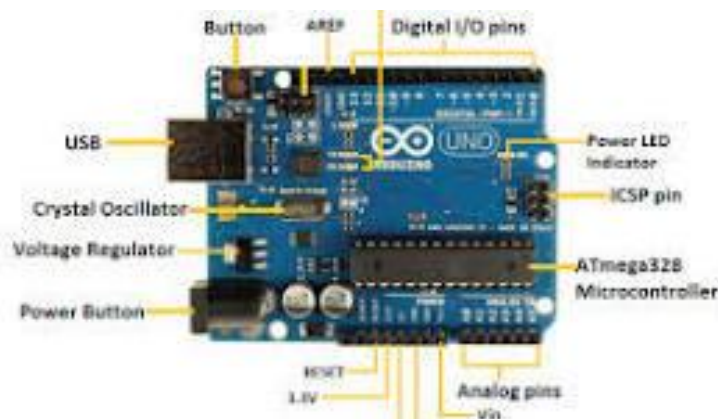
Fig 5: Hardware parts of Arduino (javaTpoint 2021)
