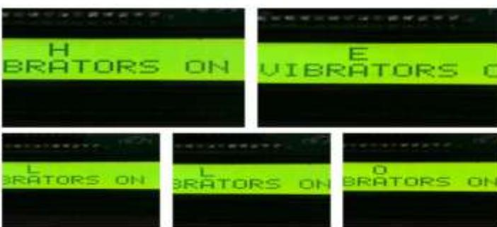
Figure 7: The SMS displayed on LCD Characters in Braille pattern
