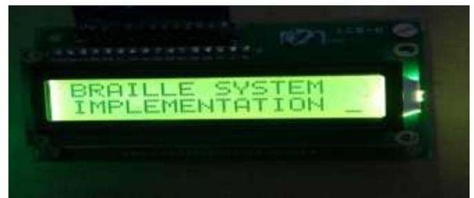
Figure 3 : BRAILLE SYSTEM IMPLEMENTATION is displayed on 16x2 LCD.
