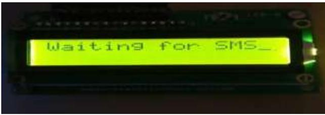
Figure 5 :System waits for SMS and it is displayed on LCD as WAITING FOR SMS.
