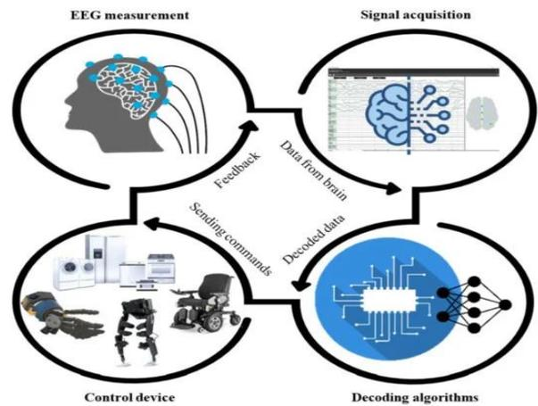
**Fig. 1. Overall architecture of the brain computer interface system**
