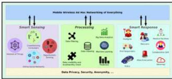
Fig -3: The proposed smart system for disaster prediction, discovery and response for smart cities [8]
