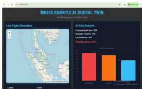
Fig. 1 – MH370 Agentic AI Digital Twin Dashboard Overview: displays live flight simulation map with animated aircraft marker, AI risk analysis panel showing Communication Failure 92%, Navigation Deviation 85%, Fuel Exhaustion 68%, and Final Risk Score 82%, with interactive Chart.js bar chart visualization.
