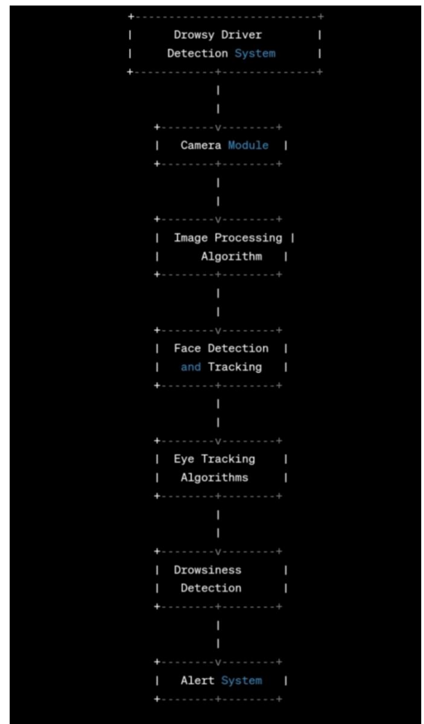
Fig 1: Block diagram of AI Base smart alert system for drowsy driver detection system
