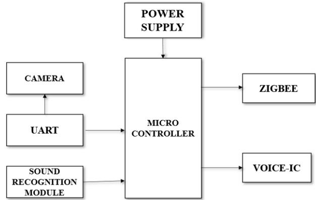
Fig:1 Block diagram for monitoring section
