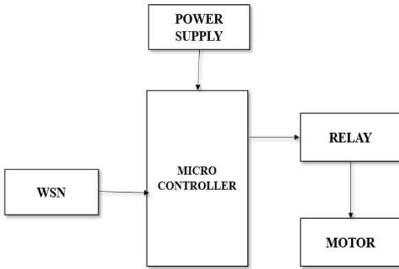
Fig:2 Block diagram for receiving section
