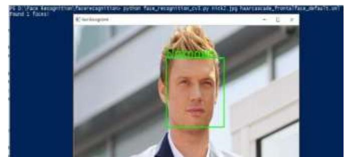
If the similarity score falls below a predefined threshold, the individual is classified as an intruder. In such cases, the system immediately initiates predefined security actions, including activating an alarm, recording video evidence, and sending notifications to the homeowner. The entire process is automated and operates continuously in real time.
