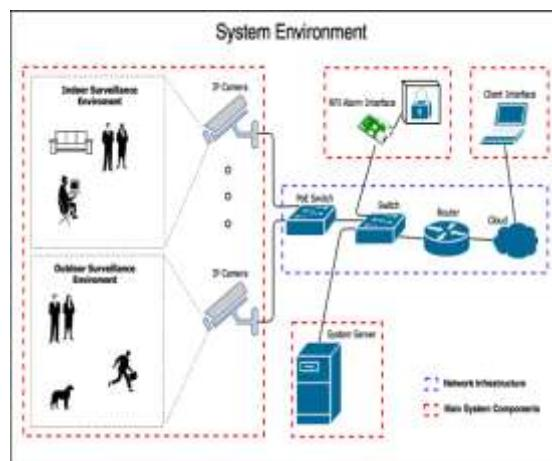
The overall architecture of the proposed system follows a layered and sequential workflow that enables real-time surveillance and autonomous response. The workflow begins with continuous video capture from the camera, which serves as the primary input to the system.
