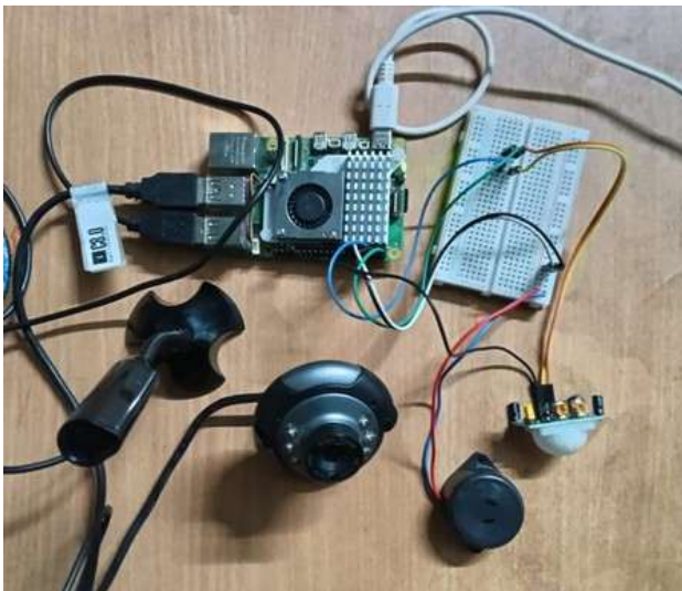
Fig. 4. Experimental Hardware Setup of the Proposed AI-Based Animal Detection and Classification System
