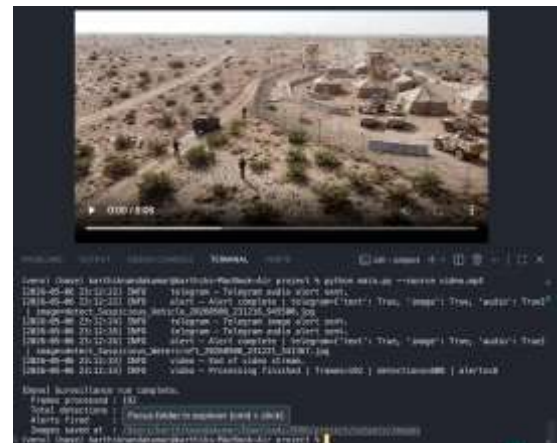
Fig 6. Video Processing Execution: Shows the surveillance system processing video frames, detecting dangers, and generate alerts on Land Terrain.
