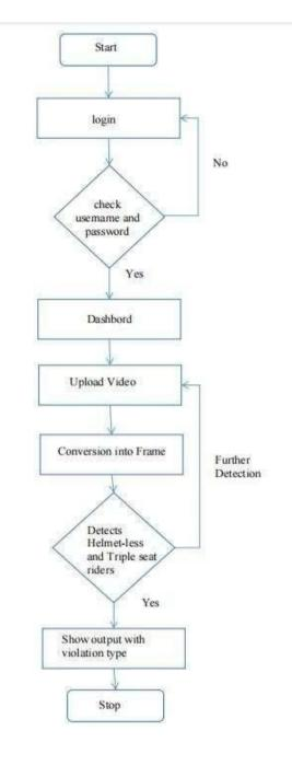
Fig -1:System Workflow
