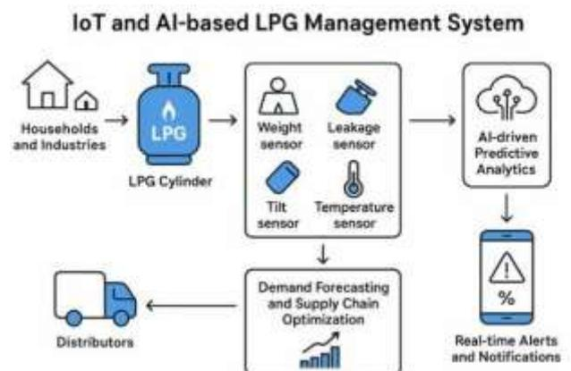
Fig. 1. 1: Block Diagram of AI-Driven IoT-based LPG Management System
