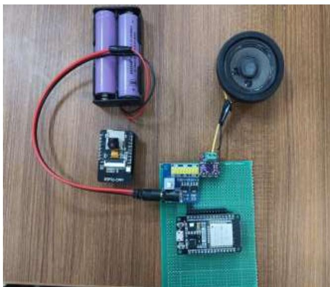
The implemented Intelligent Visual Assistant system successfully achieved its intended objectives by providing real-time object detection and voice-based feedback using a hybrid IoT and AI architecture. The ESP32-CAM effectively captured images and transmitted them to the Flask server over a local Wi-Fi network.
