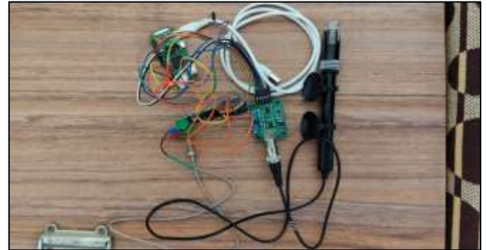
Figure 4.1: Water quality monitoring system hardware setup
