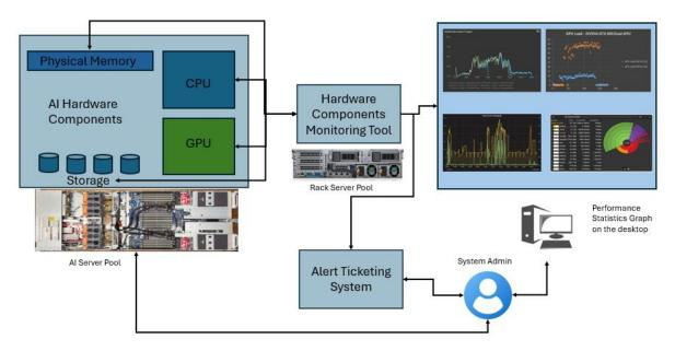
Figure 1: Monitoring model for AI system resources
