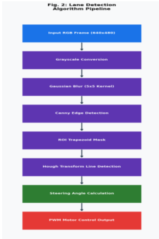
Fig. 2 (left): Lane Detection Algorithm Pipeline. Fig. 5 (right): Visual output at each processing stage — (a) original frame, (b) Canny edges, (c) detected lane lines with steering vector.
