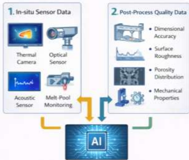
Fig-6: Sensor and Quality data as data inputs for Ai-Based DFM.
