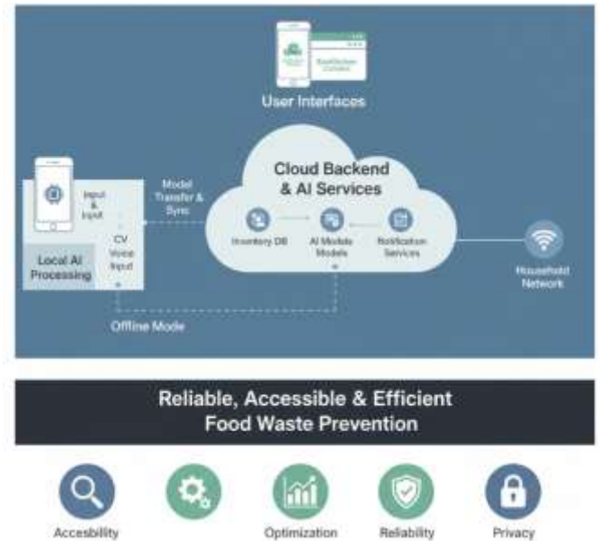
Fig. 4. Implementation Framework of EcoKitchen Connect illustrating the hybrid deployment model, on-device optimization, and accessible UI/UX components.
