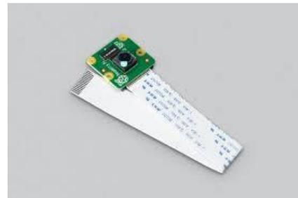
The Raspberry Pi Camera Board is a custom designed add-on module for Raspberry Pi hardware. It attaches to Raspberry Pi hardware through a custom CSI interface. The sensor has 5 megapixel native resolution in still capture mode. In video mode it supports capture resolutions up to 1080p at 30 frames per second.
