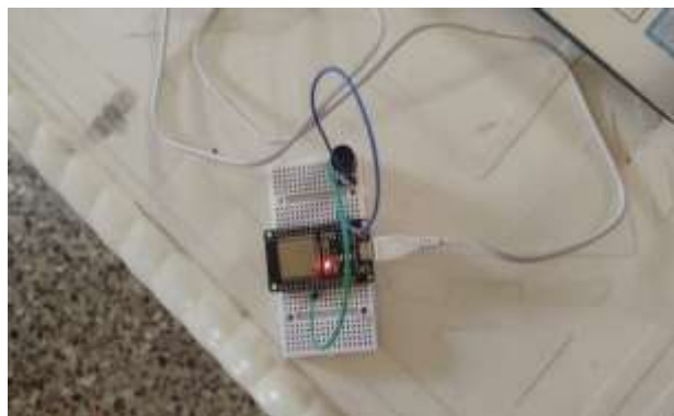
Fig 3. ESP32-Based IoT Bird Deterrence Hardware Prototype
