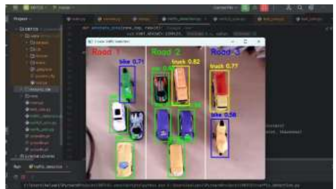
Fig-7.5: Trained YOLO model detecting vehicles
