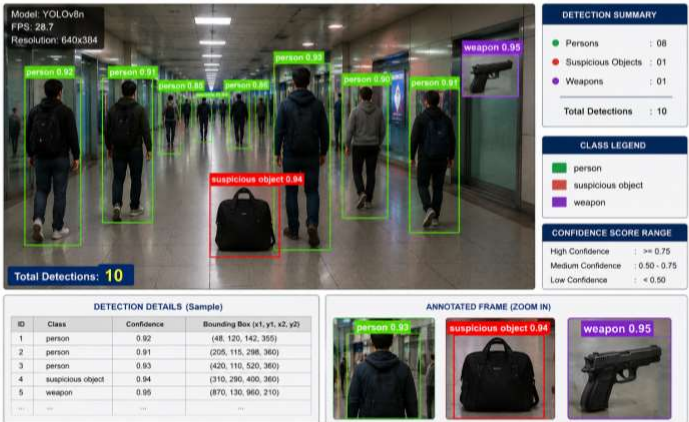
Figure 3: YOLOv8 Detection Output with Bounding Boxes
