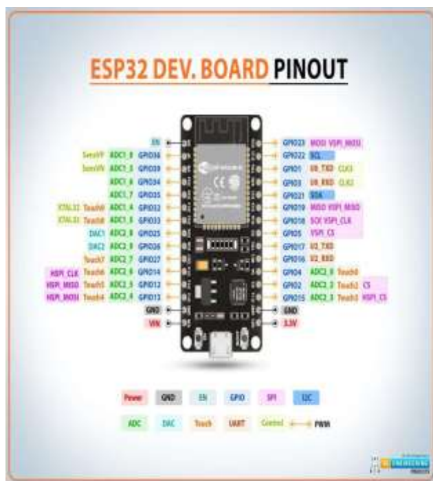
Fig. 3 ESP32 PIN DIAGRAM
