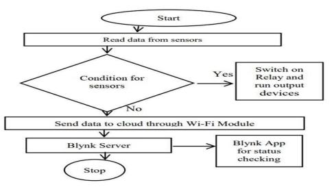
Figure 3: DFD for air pollution monitoring system
