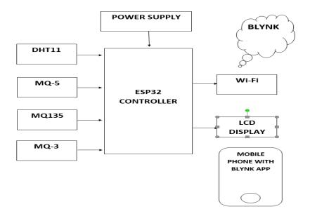
Figure 1: Block diagram for Air Pollution Monitoring System
