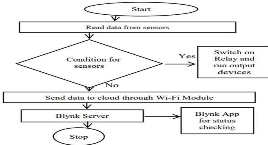
Figure 3: DFD for air pollution monitoring system
