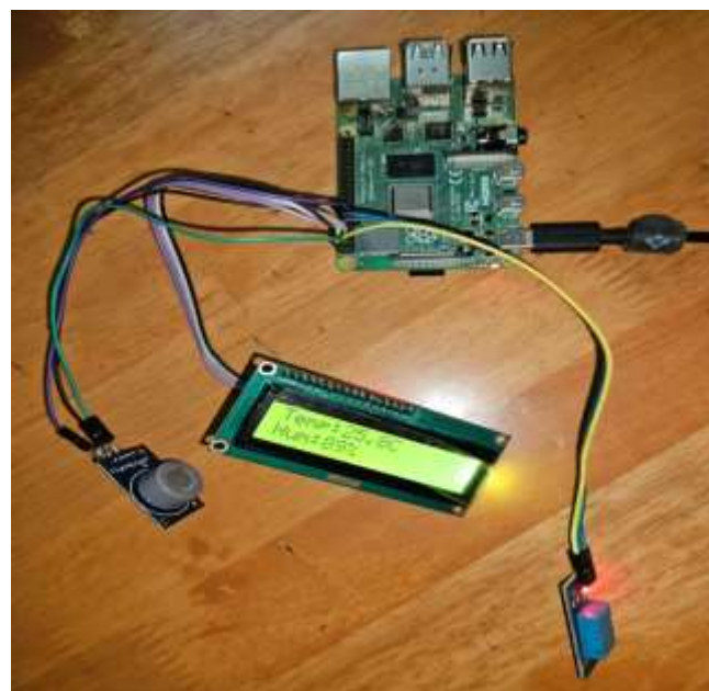
Figure 4: The hardware implementation of the designed system with temperature and humidity outputs
