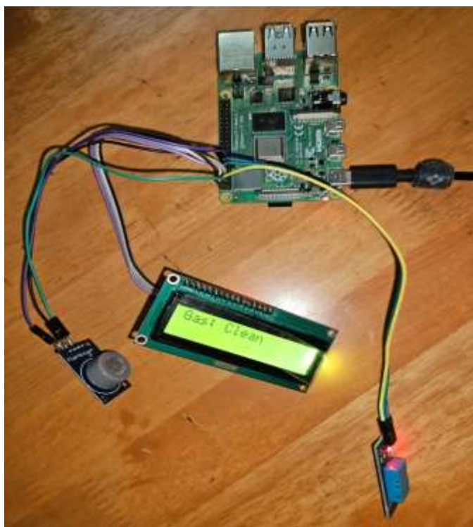
Figure 5: The hardware implementation of the designed system with Gas outputs
